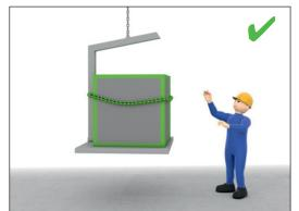
Secure the load against falling
